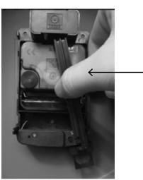
2. Hook the pendulum up to the swinger as per the picture shown.
