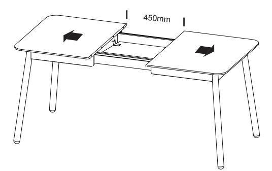
Step 3 Carefully lift the extension leaves out together as shown below.
