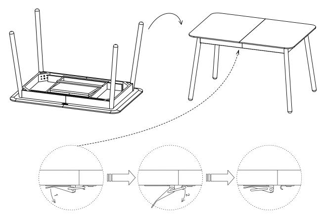
Step 2 Pull end of table to oposite direction by 2 persons, open to the end position, Open distance will be 450mm.
